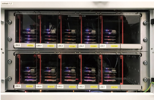
FIGURE 11. Detail of measurement equipment showing one group per UUT position to enable fully parallel test execution.
