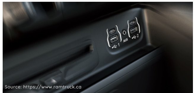
Source: https://www.ramtruck.ca FIGURE 1. A typical dash-mounted automotive USB hub module (courtesy of https://www.ramtruck.ca )
