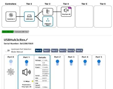
**ControlRoom** is an AV-focused application to visualize the USB tree and remotely control Acroname hubs, switches, and extenders.
