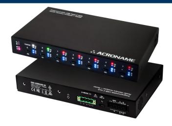
The USBHub3c is a high-performance, managed industrial USB hub featuring six USB-C ports, supporting data rates of up to **10 Gbps** and **100 W USB Power Delivery** (USB-PD) per port.
