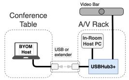
The USBHub3+ is ideal for adding bring your own meeting (BYOM) capability to your conference room. Out of the box, USBHub3+ is set to **auto-switching mode**, based on port-priority, to easily detect a connected host device and automatically switch peripherals to that host.
