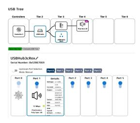
**ControlRoom** is an AV-focused application to visualize the USB tree and remotely control Acroname hubs, switches, and extenders.
