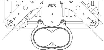
**Step 2:** Attach the mounting bracket to the Bottom Chassis Plate using the two  $#4-40 \times \frac{1}{2}$ " socket-head cap screws and #4-40 nylon-insert locknuts, and tighten with the 3/32" hex key and wrench.
