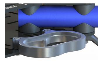
**Step 3:** Insert the SF11 laser rangefinder (as shown below) into the figure-8 shaped opening. Secure with two  $#4-40 \times 1/4"$  long, socket-head screws using the 3/32" hex key. Do not overtighten. If available, we recommend you place a small drop of medium-strength thread-locking fluid onto each screw first.
