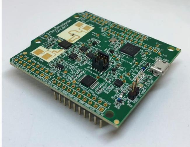
Figure 4. Basic Arduino Header Installation (Option B)
