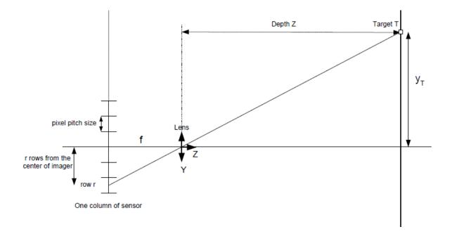
The depth distance (Z) produced by the API is the perpendicular distance from a target point to the front glass of the camera. The depth distance is different from the range distance which is the straight line distance from a target point to the camera. Note that if the target lies on the optical axis of the camera lens, the depth and range distances are the same. See picture above. The camera performs the necessary conversion from the range data to depth data for off-center targets.
