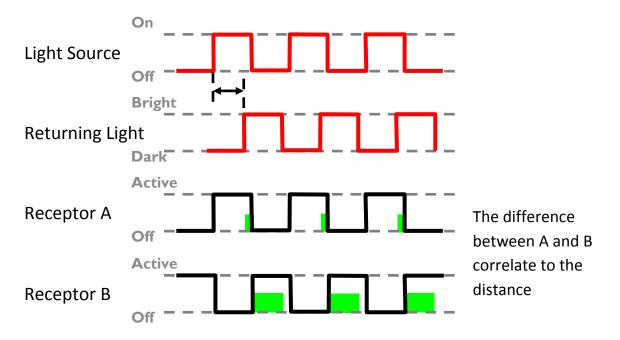
The maximum measurement distance is given by the modulation frequency.
