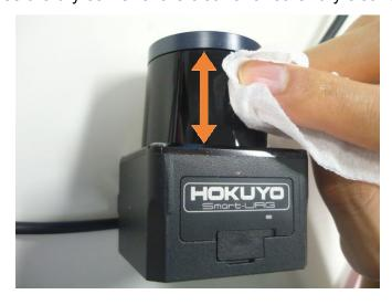
6) Check to make sure that there are no **uneven marks** caused by wet wiping. Then the cleaning process is completed.
