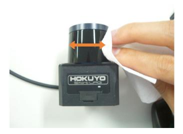
4) Remove any dirt on the bottom of the lens as well.
