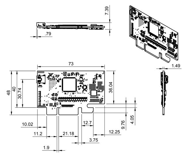
Figure 4: MTM-USBStem Mechanical
