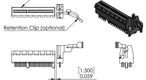
Figure 3: PCIe Vertical Connector with optional Retention Clip
