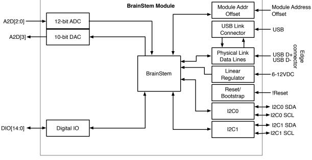
Figure 1: MTM-USBStem Block Diagram
