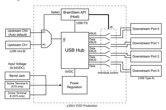
Figure 1: USBHub2x4 Block Diagram
