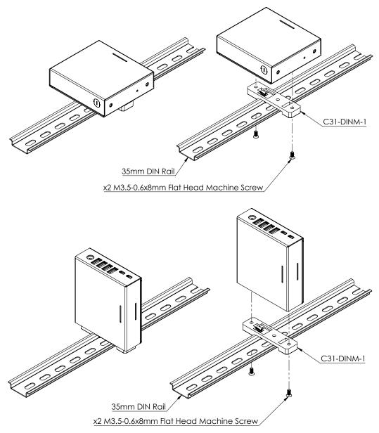
Figure 8: USBHub2x4 DIN Rail Mount
