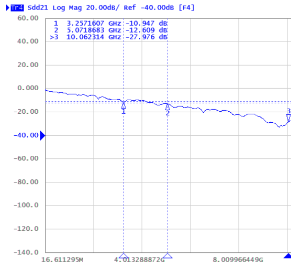
Figure 8: Typical SS data differential insertion loss
