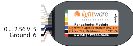
Figure 8 :: Analog voltage connections
