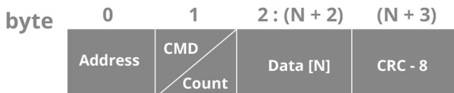
Figure 17. Frame structure for Evo Thermal commands
