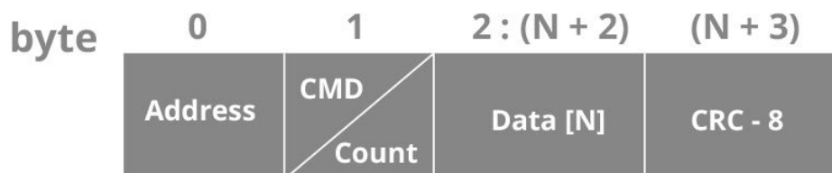
Figure 17. Frame structure for Evo Thermal commands
