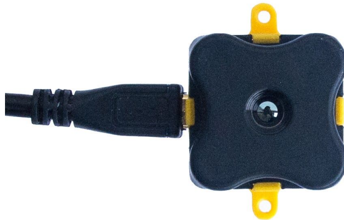
Figure 3. Module orientation for correct thermal image. Evo Thermal 33.
