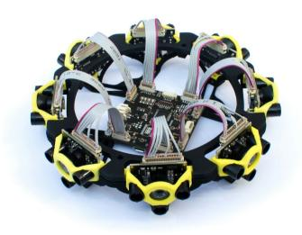
TeraRanger Tower is sold as a self-assembly kit and takes less than 10 minutes to build. A tutorial video and user manual are available on our website, and a scan format ROS (Robot Operating System) node will get you up and running quickly. A free Windows GUI is also available, allowing you to to see graphically the distance values being obtained and set certain sensor parameters with a just a few mouse clicks.
