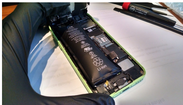
FIGURE 1. iPhone 5c damaged by swollen battery.
