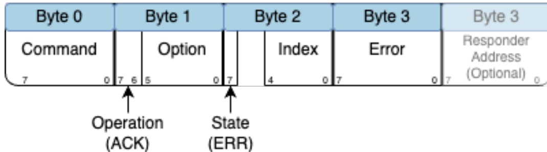
Fig. 6: Packed Byte ACK UEI Error Structure
